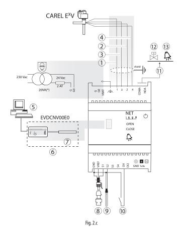
(\*) in combination with Alco EX7 or EX8 valves, use a 35 VA transformer (code TRADRFE240)
