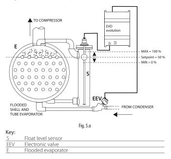
With the condenser, the action is direct: if the liquid level measured by the float level sensor is lower (higher) than the set point, the EEV valve closes (opens).
