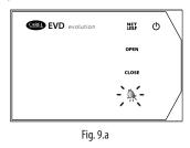
**Note:** the alarm LED comes on to signal a mains power failure only if the EVBAT\*\*\* module (accessory) has been connected, guaranteeing the power required to close the valve.
