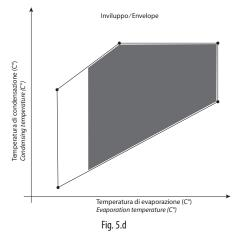
The pCO controller defines the current set point according to the point of operation within the envelope:
