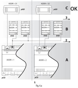
Important: if the addresses are not assigned in this way, as for example shown in the following figure, malfunctions will occur if one of the pCO controllers is offline.
