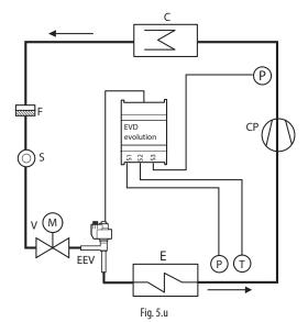
Key:CPCompressorEEVElectronic expansion valveCCondenserVSolenoid valveFFilter-drierEEvaporatorSLiquid gaugePPressure probe (transducer)TTemperature probe
